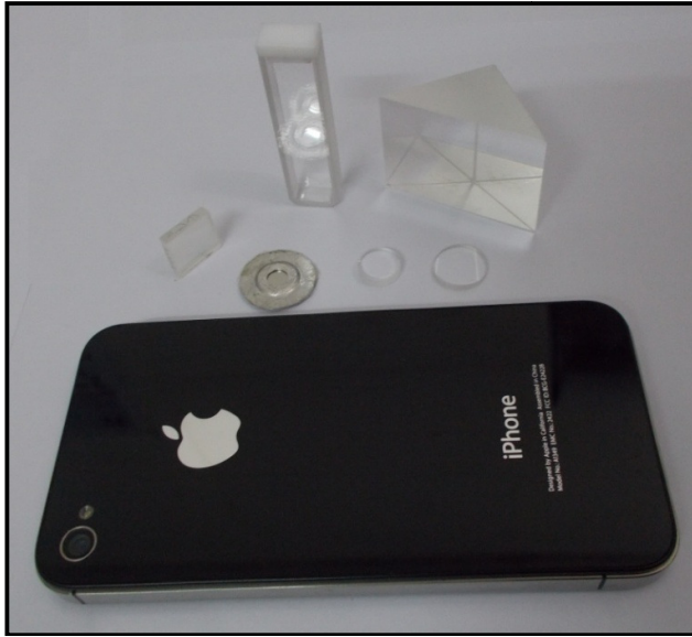
Figure 1: Optical components used in the spectrometer.
