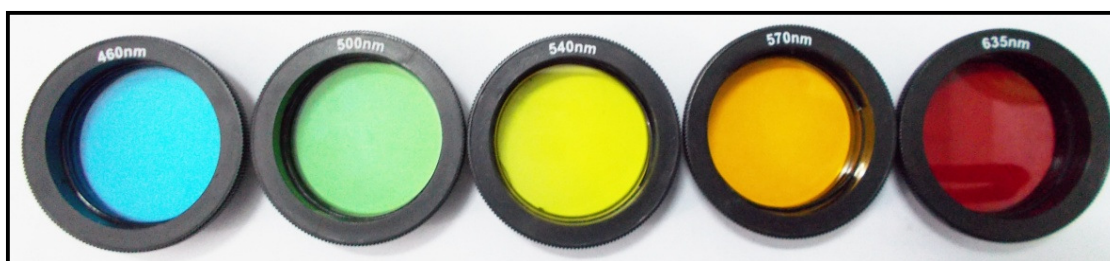
Figure 8: Photographic images of the colored filters whose absorption bands have been measured.
