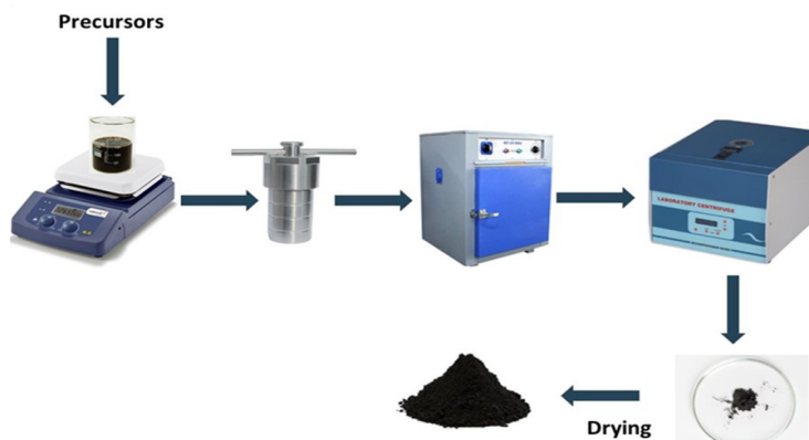
Figure 1: Schematic representation of the hydrothermal technique.
