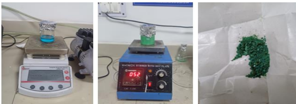
Figure 2: Camera images of (a) Stirring of precursor solution (b) Stirring of precursor and Neem extract (c) Annealed (at 250^\circ\text{C} ) and dried CuO powder.
