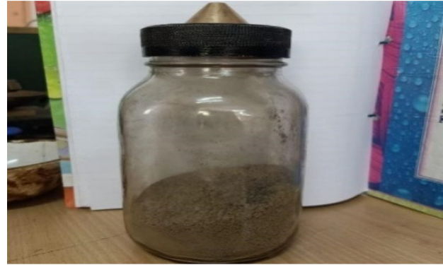
Figure 4: Pycnometer to test specific gravity Consistency's Limit Test.
