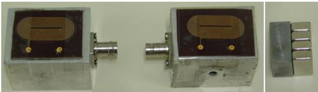
Figure 4: Photograph of the SH wave EMATs with elongated spiral coils and array of periodic permanent magnets (PPM).
