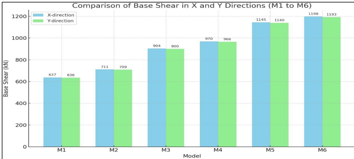
Figure 3: Base shear comparison for all models.
