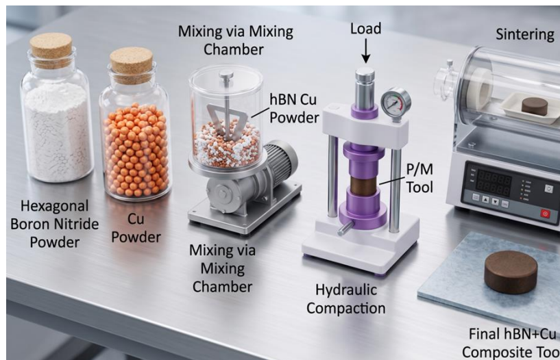
Figure 2: Powder metallurgy-based tool fabrication process and prepared hBN–Cu composite tool electrode.
